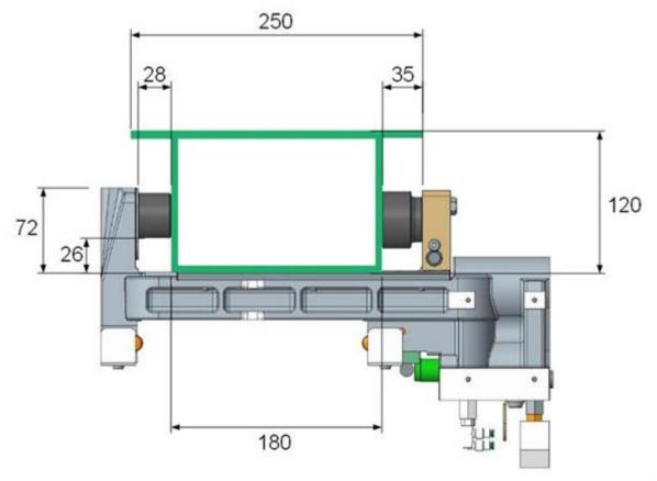
Maximum workable profile on three faces with cone + tool with 110 mm spindle end projection and work table 90°
