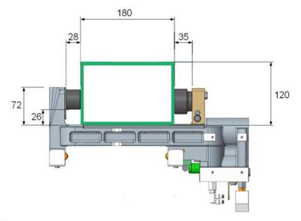
Maximum workable profile on three faces with cone + tool with 110 mm spindle end projection and work table rotation  $0^\circ/90^\circ/180^\circ$
