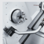
Automatic in-machine tool presetter
