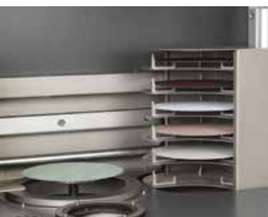
Step 1: The centre piece of the MD-Disc lifts the MD-Consumable to be replaced.
