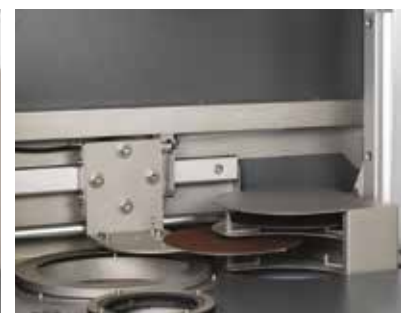
Step 4: The following MD-Consumable is taken from the elevator and moved to the MD-Disc.
