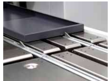
Part lined up with the squaring arm.
