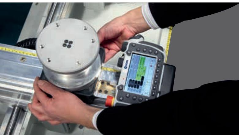
In the “Pilot” version positioning is guided and controlled by the workpiece program. Magnetic sensors detect the correct position of all components, eliminating the risk of collision.
