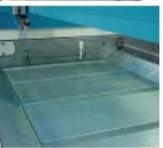
Qty (2) The steel cover is designed to avoid that the abrasive lying on the chutes slides down inside the dredge when the waterjet goes over it, causing a system overload.
