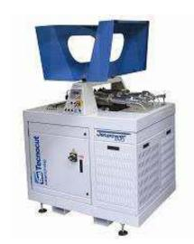
The 60 HP (45 kW) pressure intensifier is made out of **3 parallel**, synchronized and independent pressure multiplier pumps, hydraulically driven, and electronically synchronized. This technical solution assures a constant and even pressure signal at a pressure of 4130 bar.
