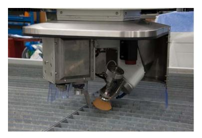
A 5 Axes Head provides 5 axes capability to the machine allowing chamfer and 3D cutting, produces more accurate parts at significantly higher cutting speeds than parts cut with conventional systems.
